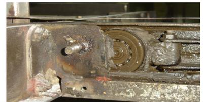
Photo of over Applying Lubricants
